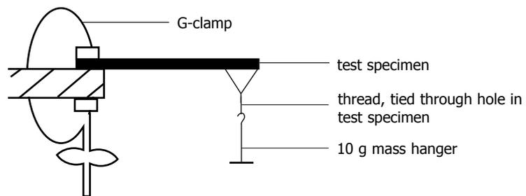
**Methods of testing joints -****Part 4: Making permanent electrical joints: soldering**
