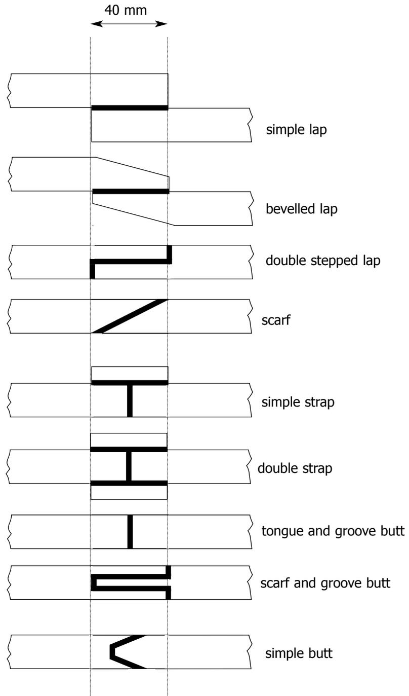
**Methods of testing joints -****Part 2: Comparing the strength of bonded joints in shear**
